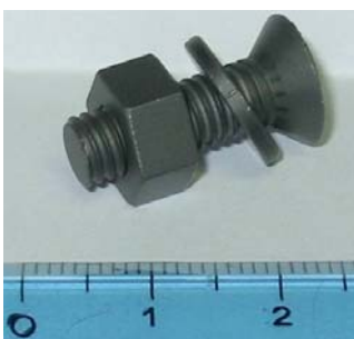
Example of complex shape obtained by EDM- electrical discharge machining- of electroconductive ceramic
