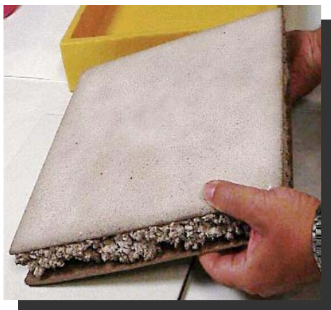
Sandwich panel for thermal insulation produced from ceramic wastes
