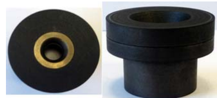
TaC nozzle prototype fabricated at ISTE
