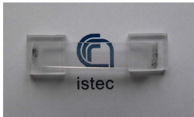
MgAl_2O_4 spinel sample prepared by hot pressing
