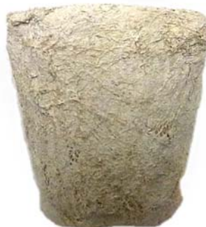
Wool-geopolymer pot and its surface structure
