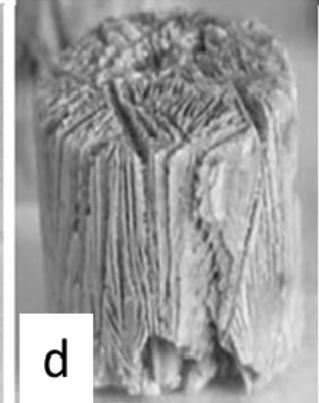
Highly porous ceramics prepared using (a) direct foaming, (b) and (c) replica technology, d) freeze casting
