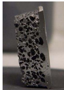
ZrB 2 based foam produced by sponge replica coupled with slip casting
