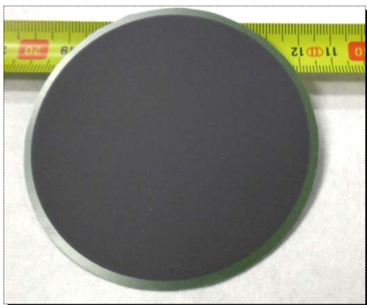
Final SOFC device (on the left) and its microstructure (on the right).
