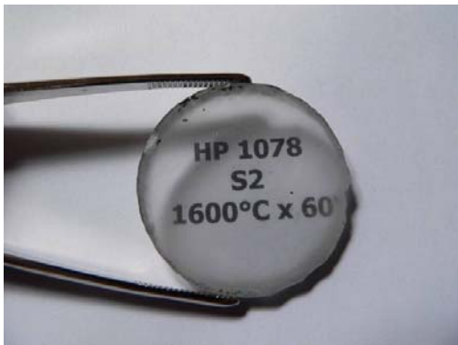
MgAl_2O_4 spinel sample prepared by hot pressing
