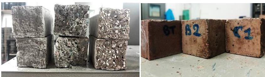
Figure 1 – RE 4 mortars: alkali-activated binders (PFA/GGBS and ceramics/GGBS blends) combined with CDW-derived aggregates (mineral fraction, rigid plastic and wood/plastic scraps).
