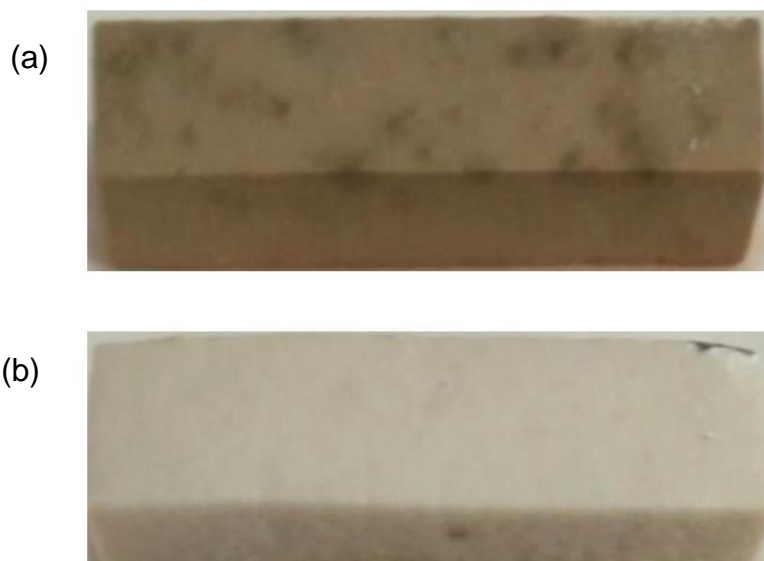
Figure 1. Prismatic specimens based on CAC50 (a) and CAC80 (b) after calcination at 1450°C overnight.
