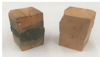
Figure 2: Adhesion test on commercial bricks with concrete and with AA concrete
