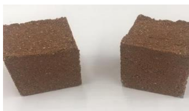
Figure 1: AA bricks made from CDW with uniaxial pressing
