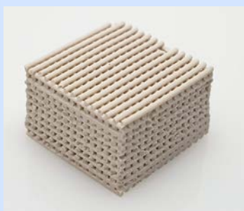
Fig. 1 Optical micrographs of 3D-printed geopolymer lattices prepared by direct ink writing.
